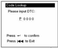
You can use  $[\uparrow][\downarrow]$  key to change P letter. And press  $[\blacktriangleleft]$  move the cursor to right. And then press  $[\uparrow][\downarrow]$  key to input number. After you input the code number, press  $[\blacktriangleleft]$  to view the definition of the code. After viewing the definition, press  $[\blacktriangleleft]$  to return the Main Menu.
