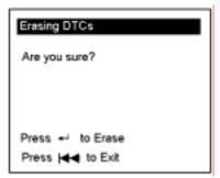
Press [ ] to erase DTCs, and the screen will display the interface as shown below:
